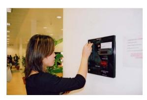
The EP7100 QubeLoader is a simple way for staff to credit their accounts. It is specifically made to take cash payment (coin or notes) and load it into the user's account. It works like a bank cash machine, only in reverse. With this loader, the card is simply presented to the reader and coins and/or notes loaded into it. This amount is then added to the account. The bright, fluorescent read-out will verify the new balance. Units can be sited at a central point or
